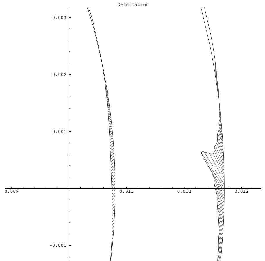
Figure 2: Surface and subsurface displacements due to a concentrated load applied at 45 degrees to the surface. It is assumed that \mu_f \geq 1.0 . The dashed lines are drawn between the undeformed and deformed positions. The units are meters. The center of the cylinder is located far off to the left hand side of the page.
