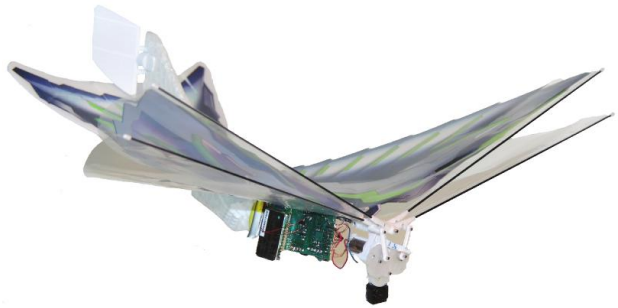
Fig. 1. The modified 12 gram flapping wing robot with custom made electronics.
