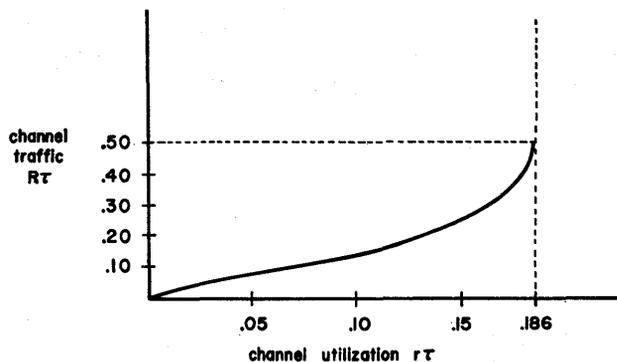
Figure 3—Channel utilization vs channel traffic
