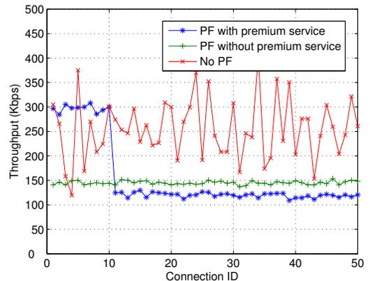
Fig. 5: Fairness test (throughput of individual connections)
