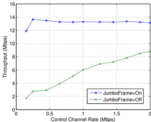
Fig. 4: Effect of control channel rates(8 data channels of 2Mbps)
