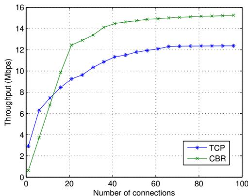
Fig. 7: System throughput(1 control 8 data channels of 2Mbps)
