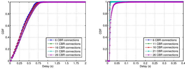
Fig. 6: Delay CDF of TCP (top) and CBR (bottom) (8 data channels of 2Mbps)
