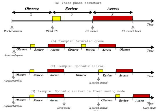
Fig. 1: Asynchronous Split Phase
